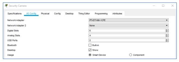
b. Attach the security camera to the wired network.
